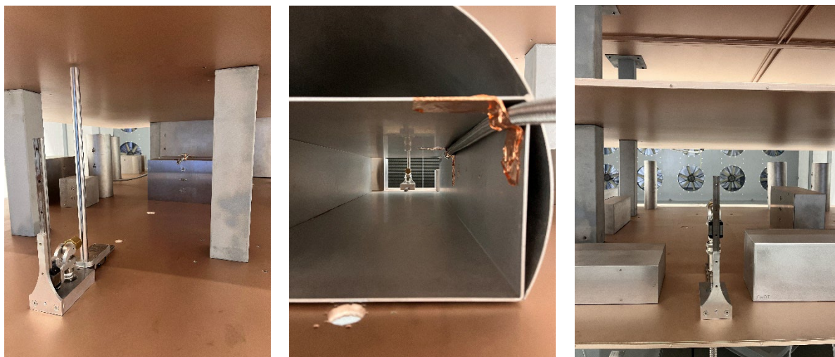
Figure 4: Different configurations for sensor testing: Urban, Tunnel and High Atmosphere
