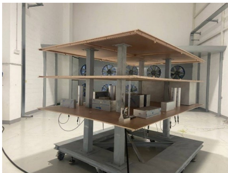
Figure 2: Mock-up for hydrogen releases in the wind tunnel
