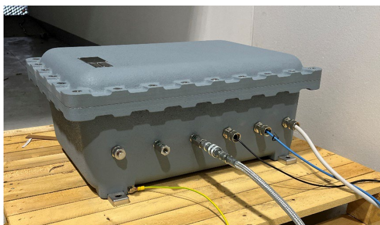
Figure 3: AUTOMA sensor casing and connections
